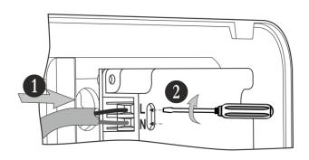
**ATTENTION:** The wires should be placed tight in the socket terminals!
