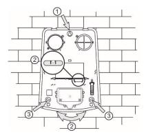
4. Set the tamper position as use the screw on it regulate the position so that the screw end to contact
