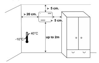
**ATTENTION:** The control panel installation location should be dry and should not be subjected to harsh temperature changes. The control panel should be installed close to grounding and telephone cables.
