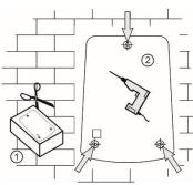
3. Mount the siren's base as first fit the screw for the main installation hole, then level the siren, and at the end fix the supporting screws on the both sides.
