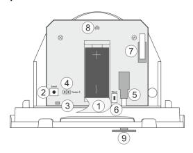
1 - Protection folio for the battery on the main board; it is removed directly before the enrolment of the detector to the panel. The other two batteries are located on the second board behind the PIR part.
