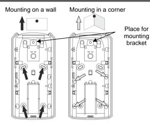
ATTENTION: When the detector is installed on a mounting bracket, it is impossible to use the second tamper-switch for self-protection (on the back side of the PCB) and the requirements of standard EN50131 Grade 2 are not covered!
