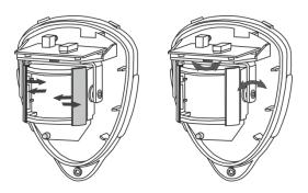
According the application you can mask sections from the lens so to obtain maximum efficiency in operation – see also the examples for the beam coverage diagrams.
