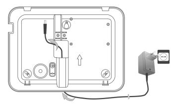
The cable length of the power adapter is ~1700mm, so you have to locate the panel installation place near a power socket.
