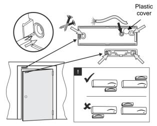
**Note:** To use the wired zone input you have to drill an additional hole for the cables.
