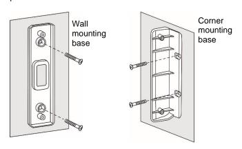
Mount over the base the detector's back box using the 2x10mm screws.
