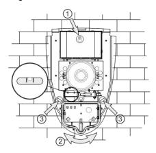
5. Set the tamper position as use the screw on it — regulate the position so that the screw end to contact with the installation surface, and the contact plate to be pressed when the cover of the siren is closed (the plate must be horizontal and when pressed with siren cover to close the tamper button under it — a click is heard).
