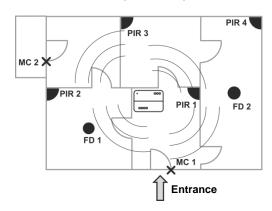
The minimum distance between the panel and enrolled peripheral devices must be 1 meter to guarantee the proper operation of the system, including in test mode.
