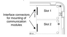
ATTENTION: The communication modules must be added to the system configuration ONLY WHEN both main power supply of the control panel and back-up battery are SWITCHED OFF. The communication modules must be enabled for operation via ProsTE software or Ajax SP web application.
