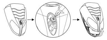
2. Remove the light pipe, undo the screws and remove one by one the metal and the plastic covers protecting the battery and the electronic parts.
