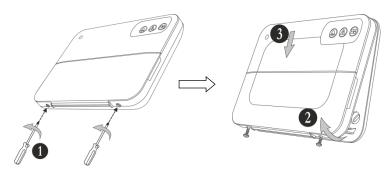
Mount the bottom of the box as use appropriate fixing elements according the mounting surface.
