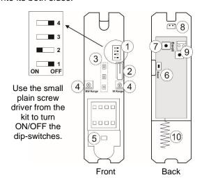
1 - Dip-switches for special functions:
