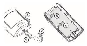
3. Mount the base of the detector's box at the place of installation. Use the respective opening according the mounting location - on a wall or in a corner.
