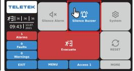
In case of Operation in Network, turn off the buzzer as choose:
