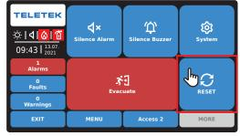
The panel is reset to Normal operation mode.
