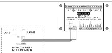
To activate the devices to be controlled, use the relay outputs 1 to 8, corresponding to the activations R1 to R8 of the monitor control screen. Relay outputs 0 and 9 are not used.
