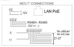
**LAN:** Ethernet connector to the building's LAN PoE installation.
