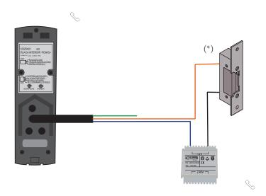
(\*) Important: Place a varistor directly over the door opener connection terminals.
